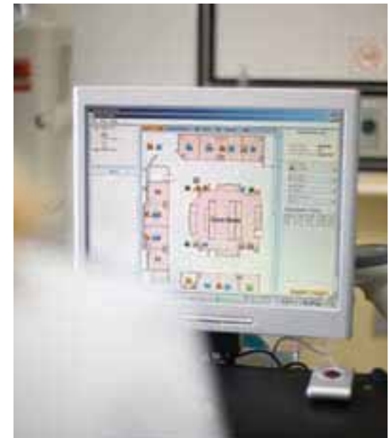
Figure 3: Searching for equipment can occupy a significant amount of nurses' time; real-time location systems (RTLS) ensure that key equipment can be rapidly located
