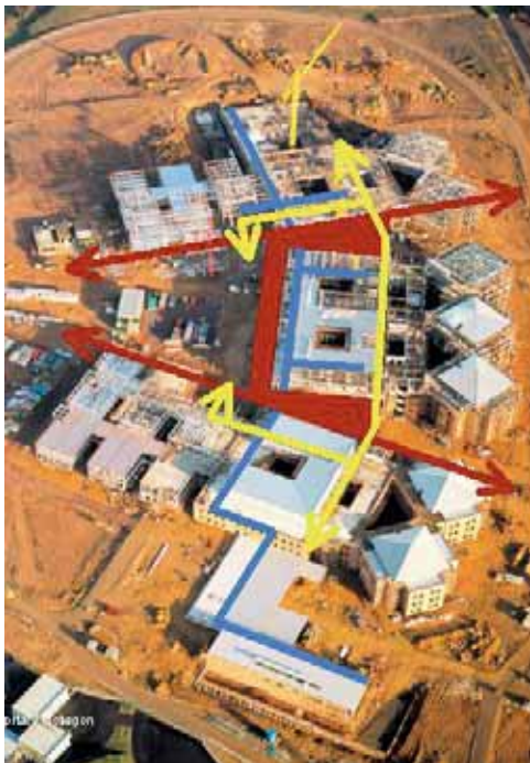
Figure 10 Composite diagram of circulation routes shows separate flows for public, patients and staff, and service traffic.
