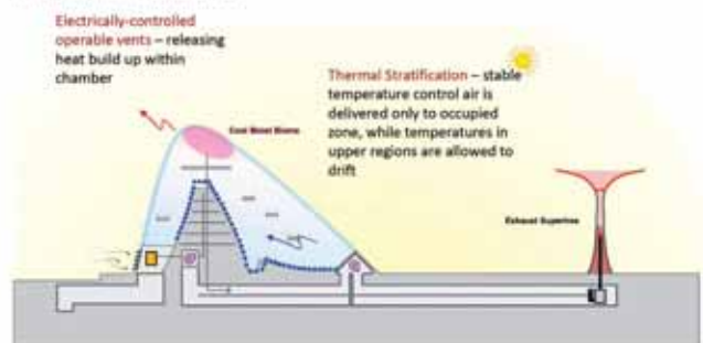
Ground cooling – chilled water pipes within concrete slab to provide radiant cooling and allows cold air to hug the ground.
