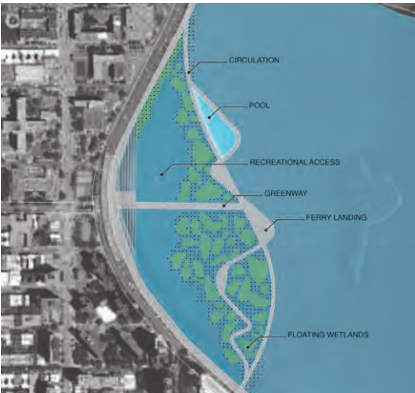
Figure 5: Within a protective cove, pilings create a dynamic neighbourhood centre with recreational access, floating community gardens and links to public transportation
