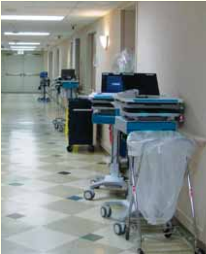
Figure 4: Hospitals should anticipate storage needs and provide easily accessible storage space, including space for computers on wheels, soiled baskets, isolation storage carts and advanced-cardiac life-support carts
