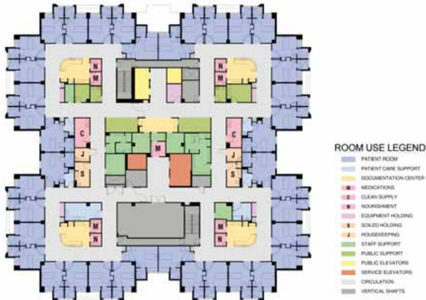
Figure 2. Bon Secours St Francis Hospital, in Charleston, South Carolina, with its unique pod design and outboard toilets, offers patient visibility through satellite nursing stations located close to the patient room
